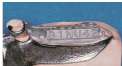
Fig. 4 The cast framework of the partial denture made from Ti-6Al-7Nb alloy. The embossed letters were clearly reproduced.
